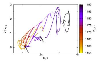
FIG. 5. Time-evolution of a jet. Solid: constant  $f_e/f_{e,max} = 0.375$  contours. Dashed: orbits of two test particles. The mass ratio is  $m_i/m_e = 4$ .
