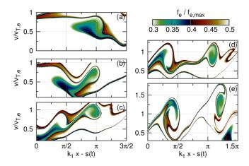
FIG. 4. Jet formation. Snapshots at  $\omega_{p,e}t = 1100$  (a), 1120 (b), 1140 (c), 1150 (d), and 1160 (e) of the electron distribution  $f_e$  (mass ratio  $m_i/m_e = 4$ ). The horizontal coordinate is shifted by  $s(t) = 0.05\pi(\omega_{p,e}t - 1090)$  in order to compensate for free-streaming.
