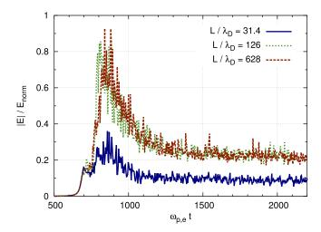
FIG. 13. Time-evolution of electric field amplitude, normalized by  $E_{\text{norm}} = m_e v_{T,e} \omega_{p,e}/e$  for different system sizes, which are indicated in the legend. Mass ratio is  $m_i/m_e = 4$ . Initial drift is  $v_d = 2.1 v_{T,e}$ .
