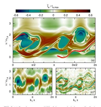
FIG. 3. (a) Snapshot at  $\omega_{p,e}t=1180$  of the perturbed electron distribution  $\tilde{f}_e$ , normalized to  $f_{e,\max}=f_e(v_{0,e})$ . Solid curve: contour of constant  $f_e/f_{e,\max}=0.375$ . (b) Low-pass filtered  $\tilde{f}_{e,\text{holes}}$ . (c) High-pass filtered  $\tilde{f}_{e,\text{jets}}$ . The mass ratio is  $m_i/m_e=4$ . The system size is  $10\pi\lambda_D$ .
